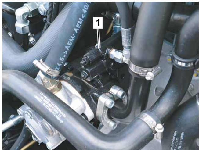
1 Hydraulic pump (variant with through-drive for power steering pump, additional steering axle)
