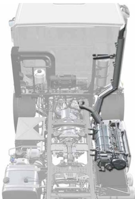
Exhaust system, upwards tailpipe (K7A)
