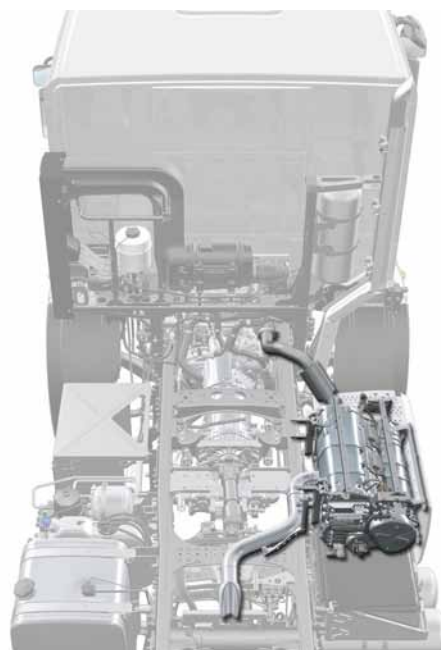
Exhaust system on right of frame, inward tailpipe (K7I)
