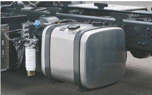
Main tank 200 l, aluminum (K0Z)
