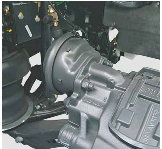
Parking brake, additional on front axle (B2Z)
