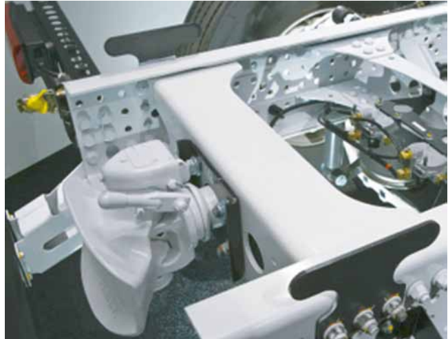
End crossmember, bolted (Q80) with standard trailer hitch, D40, Rockinger (Q7K)
